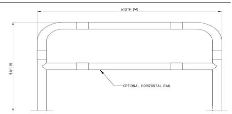
The range of Black & Yellow products are ideal for providing high visibility protection in both internal and external warehousing environments. All products in the range are galvanised mild steel, ensuring their longevity and are designed to take the knocks and bumps that occur in all warehouses.
