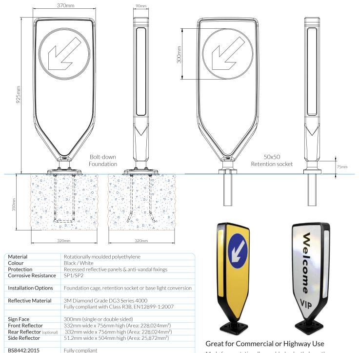
Made from rotationally moulded polyethylene, the non-illuminated sign face of the Evo-N bollard can be overlaid with any regulatory traffic sign for on highway, or any commercial design for car parks and business sites. And like the rest of our traffic bollards the Evo-N can be single or double-sided.
