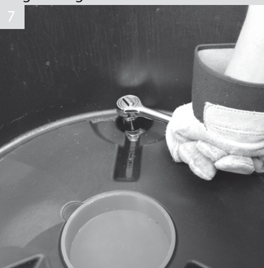
7 Use a spanner or socket to tighten the bolts
